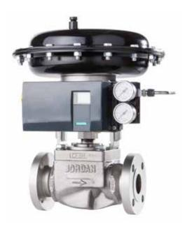
The Mark 78 Series is designed for accurate performance and simplified maintenance. This versatile product can be used on a variety of applications including viscous/corrosive liquids, process gases or steam in process or utility service. The top entry cage design allows maintenance while the valve is in the line. Characterized flow options including linear, equal percentage, quick opening or an equal-linear combination.
