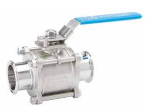
The FB8904 Series is a three-piece 3A approved sanitary ball valve with 316L construction. It is ideal for clean utility applications and the Food & Beverage and Consumer Health & Beauty industries. This valve is cavity-filled to minimize media collection. Sanitary clamp ends are standard. The inner diameter of the end connections is the same as the ID of the ball ensuring no obstruction of flow from inlet to outlet.
