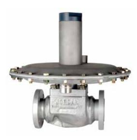
The Mark 608 Series gas pressure regulator is used on large tank blanketing applications or other low pressure gas regulation. In tank blanketing applications, the Mark 608 is used to control the flow of the blanketing gas into the tank to maintain the proper positive pressure. Once the blanket has been established, a small flow of nitrogen is continually admitted to the tank to keep the blanket fresh.
