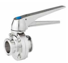
The manual FB7904 Series is a sanitary butterfly valve with clamp-ends and stainless steel body with EPDM (or Viton) seats, seals and 12 position stainless steel handle. Ideal for Food & Beverage and Consumer Health & Beauty industries. The valve is ideal for CIP/SIP, sanitary pump skids, batch processing, mixing and backflow prevention.
